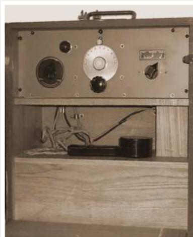
Battery-operated 2-valve transmitter/receiver.
