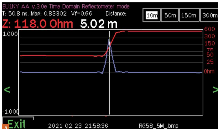
For this to work correctly, the Velocity Factor (Vf) of the cable must be known and entered into the unit. The unit is pre-set with a value of 0.66 (such as for RG58). This may be altered and stored, either temporarily or permanently. I found this feature accurate although; with some cables, the analyser presented some odd impedance values directly at the cut-off point (Fig. 5).
