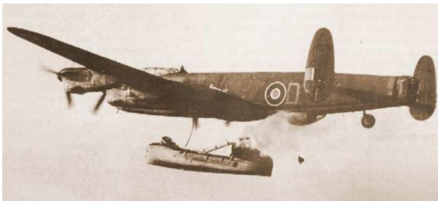
Fig. 1: Airborne lifeboat designed by Uffa Fox.
